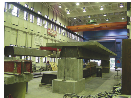
Fig. 4 With the concrete deck in place, several sections of a folded plate girder bridge can be stacked and shipped to the site on one trailer.
